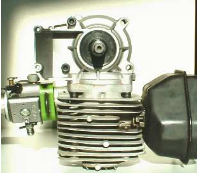
FIGURE 1 shows the G62 with all of its original ignition system removed. NOTE the two socket head cap screws have also been removed from the right side of the crankcase.
